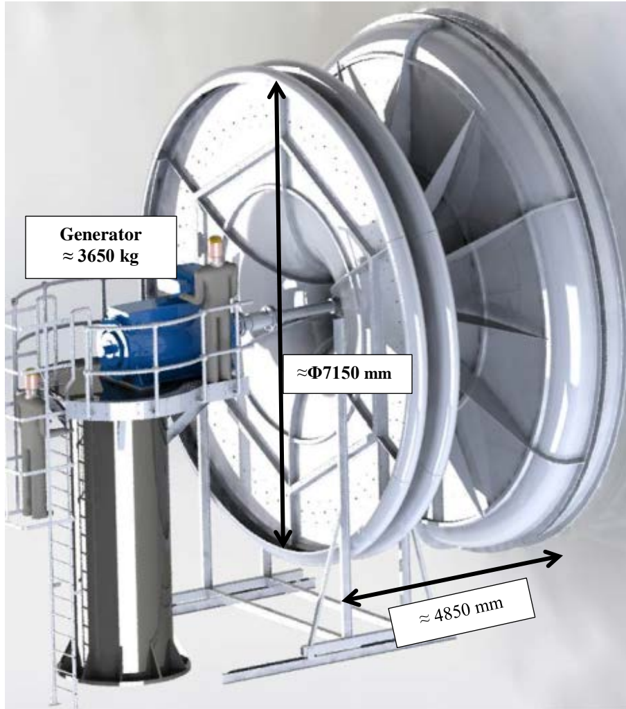
Figure 3 - HydroAir PTO Concept
